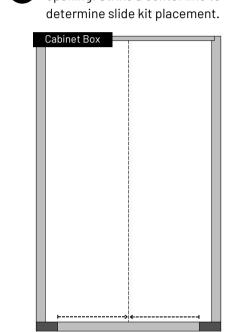
Align slide kit center markings with center line. Screw slide kit to cabinet floor with four #8 washer head screws (not provided). Slide depth placement: • Over lay doors: 1/8" back from front of face (pictured below) • Inset doors: 1/8" back from back of door when closed ace Frame Fron Mounting
