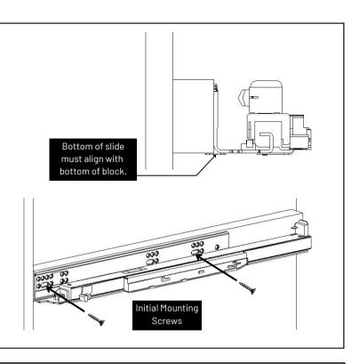
Place unit on the slides and ensure proper fit.
